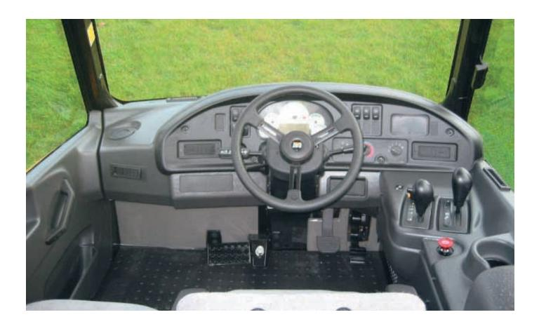
**Ergonomic Layout.** The controls and layout of the cab are designed to make it as easy to operate as your car. Quick and easy to read and simple to operate, the controls and gauges on the 730 allow the operator to concentrate on production.
